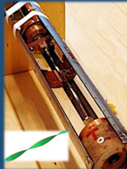
Combined torsion + tensile axial stress
